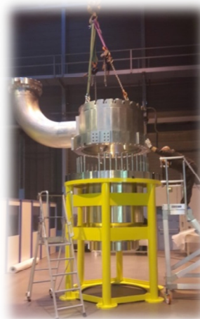
Fig. 4: Core block assembly in factory
